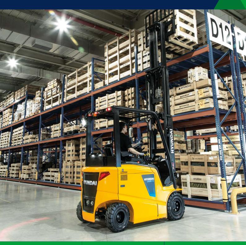
Load Capacity 1600 – 2000 kg Drive Motor Rating 9 kW
