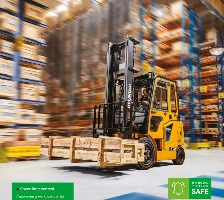
A maximum travel speed can be set to meet the safety speed of the site through a multifunctional monitor. Even when maximum speed is limited, gradeability and lifting performance are maintained at top levels.
